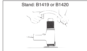
Bending and welding of PVC pipes
