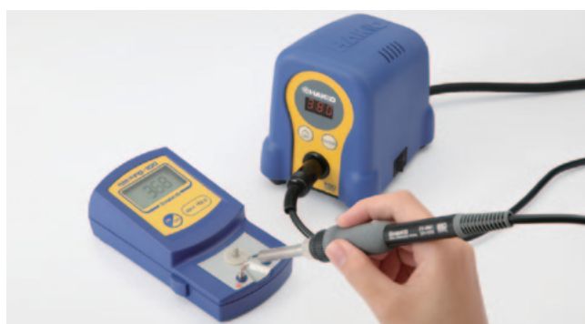
Measuring the tip temperature with a tip thermometer (HAKKO FG-100)
